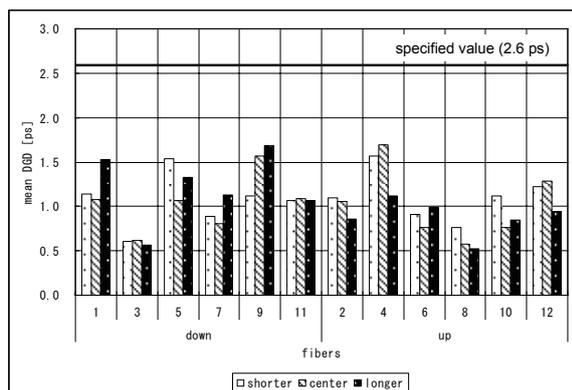
Figure 4: Measured mean DGD
