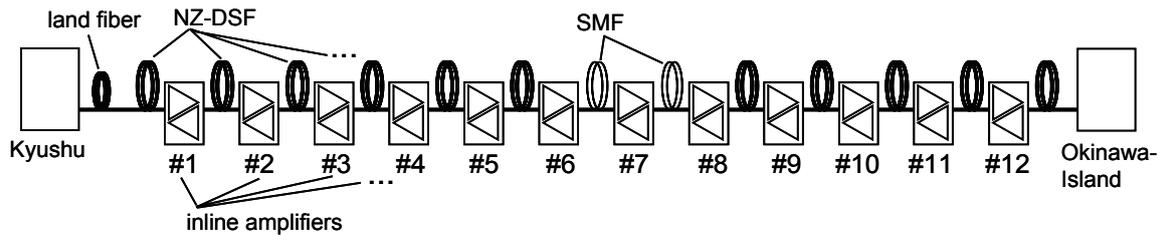
Figure 1: 900-km submarine transmission facilities
