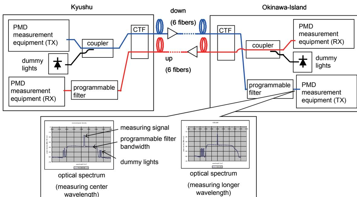
Figure 3: PMD measurement setup
