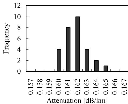
Figure 2: Distribution of attenuation of improved Z-PLUS Fiber
