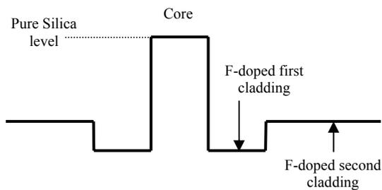
Figure 1: Schematic of Refractive index profile
