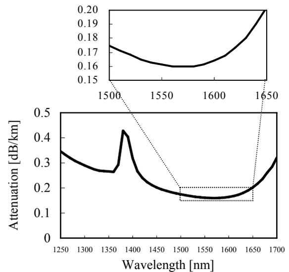
Figure 3: Typical attenuation spectrum of improved Z-PLUS Fiber
