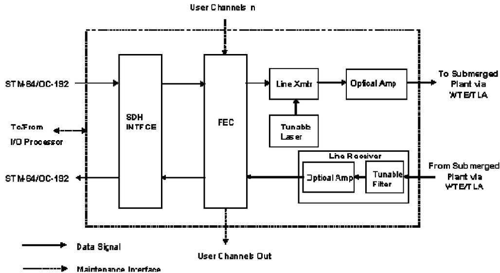
Figure 1 Functional Block Diagram of HPOE
