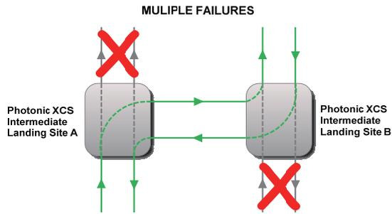
Figure 4 The network configuration in the form of an ‘H’: normal operation, and restoration with photonic cross-connects after multiple failures.
