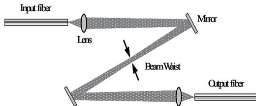
Figure 1 Simple fiber-to-fiber relay system.
