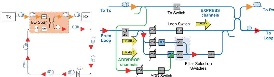
**Figure 2: A configuration of re-circulating loop with I/O span contained in shaded box is shown on left; detailed configuration of I/O span is shown on right.**
