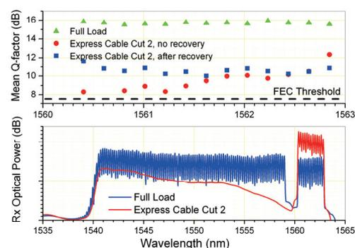
**Figure 4: Add/drop path performance data and spectra as detected at Station C.**
