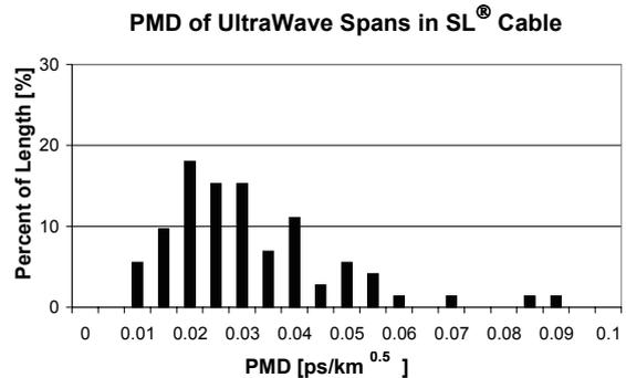
Fig.7. PMD of approximately 5000 km of UltraWave fibers in SL<sup>®</sup> cable. Average cabled PMD is 0.031 ps/km<sup>0.5</sup>. The average DGD for the LMC samples of SLA and IDF are 0.019 ps/km and 0.045 ps/km, respectively. Combining the associated LMC PMD values yields an average fiber PMD of 0.034 ps/km<sup>0.5</sup>.
