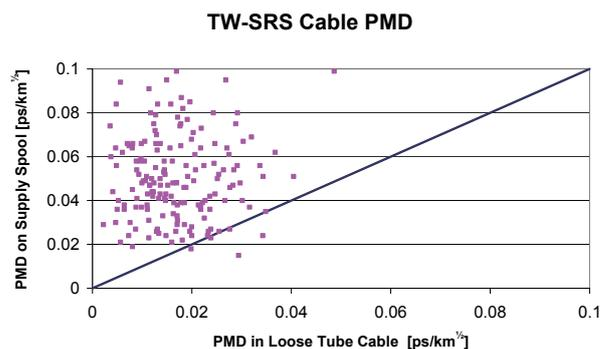
Fig. 1. Comparison between PMD as measured on the supply spool and PMD in the cable. There is no correlation between the two due to the winding tension and the bend diameter of the fiber on the spool. It is worth noting though that almost all spool PMD values are higher than the cabled PMD.
