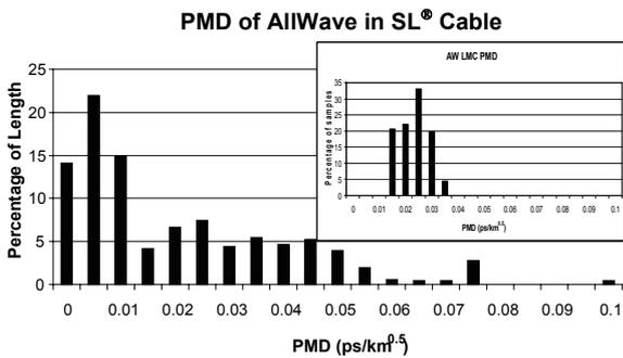
Fig.6. PMD of 7800 km of AllWave compensation fibers in the SL<sup>®</sup> cable. The RMS average cable PMD is 0.030 ps/km<sup>0.5</sup>. The insert shows the LMC PMD distribution of the AllWave fibers. The average LMC PMD is 0.021 ps/km<sup>0.5</sup>.
