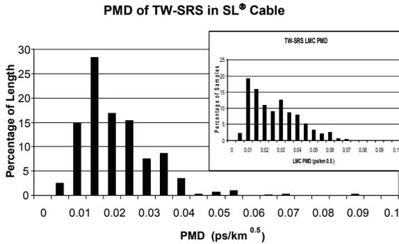
Fig.4. PMD of approximately 13,700 km of TW-SRS fiber in the SL<sup>®</sup> cable. The RMS average cable PMD is 0.021 ps/km<sup>0.5</sup>. The insert shows the LMC PMD distribution of these TW-SRS fibers. The average LMC PMD is 0.022 ps/km<sup>0.5</sup>.
