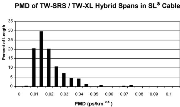
Fig.5. PMD of approximately 16000km TW-XL and TW-SRS hybrid spans in the SL<sup>®</sup> cable. The RMS average cable PMD is 0.031 ps/km<sup>0.5</sup>. The average LMC PMD of the TW-XL and TW-SRS fiber is 0.031 ps/km<sup>0.5</sup> and 0.024 ps/km<sup>0.5</sup>, respectively.
