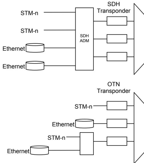
Figure 2: Comparison of SDH and OTN architectures.
