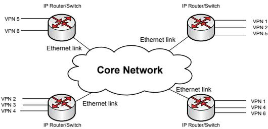
Fig 4: Basic IP-VPN Network. Virtual Private Networks are created to provide private networks within the core network. Any router can be configured with a VPN to allow the VPN owner access to that location.
