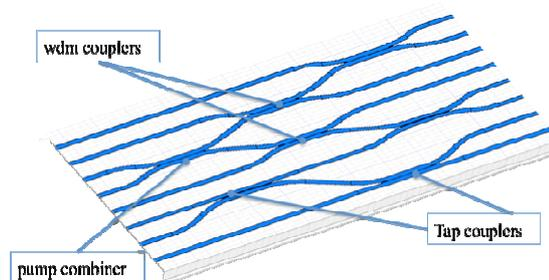
Figure 3 – Layout of the PIC for the bidirectional amplifier with loopback
