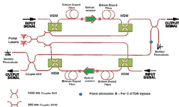
Figure 1 – Submarine optical amplifier schematic
