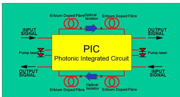
Figure 2 – Submarine amplifier schematic using PIC
