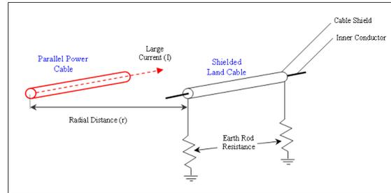
**Figure 4: Land cables connected to earthing rods**
