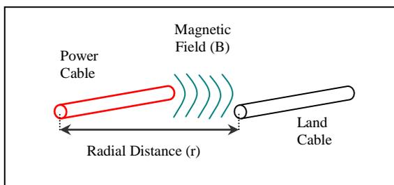
**Figure 3: Illustration of Magnetic Field (B) when a current flows through the Power Cable**
