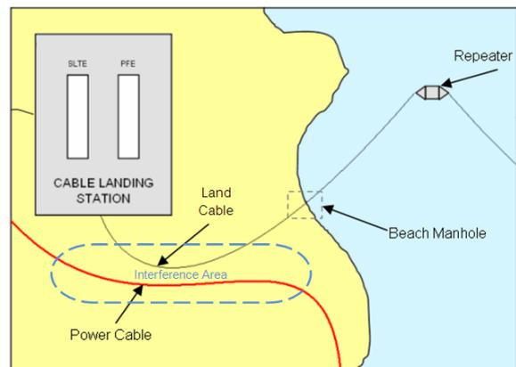
**Figure 1: High level view of cable landing and interference area of interest**
