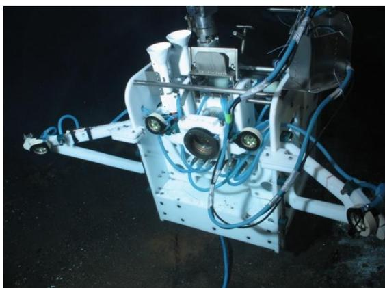
**Figure 2: Instrument dedicated to imagery and physico-chemical data, used on EMSO Lucky Strike Azores site and Neptune Canada Endeavour site. (copyright Ifremer).**
