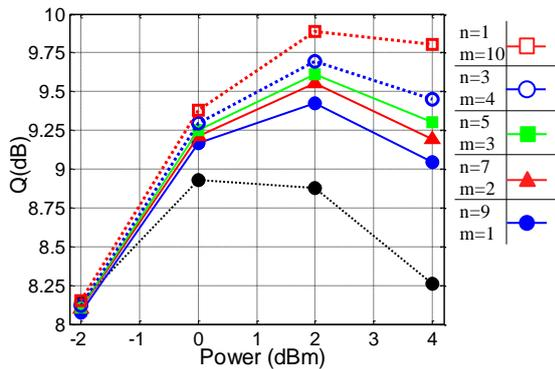
**Fig. 4:** Performance results as a function of optical power for different configurations of number of sub-bands,  $n$  and number of steps  $m$ .
