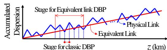
Fig. 1: Equivalent link DBP concept showing the reduced number of stages required for DBP when equivalent link is used.
