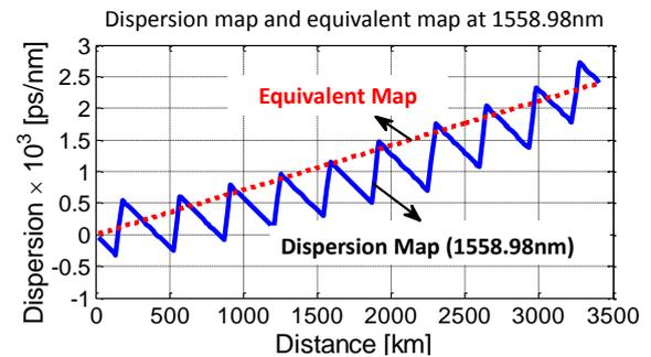
**Fig. 3: Physical dispersion map and equivalent link for DBP.**
