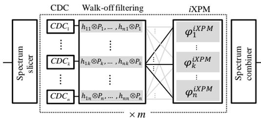
**Fig. 2: Schematic diagram of the *i*XPM back-propagation algorithm. Extension to two polarization case is straight-forward.**
