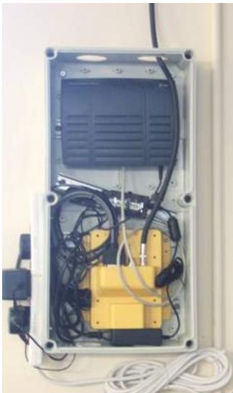
Figure 5 - AIS Receiver, data converter and modem
