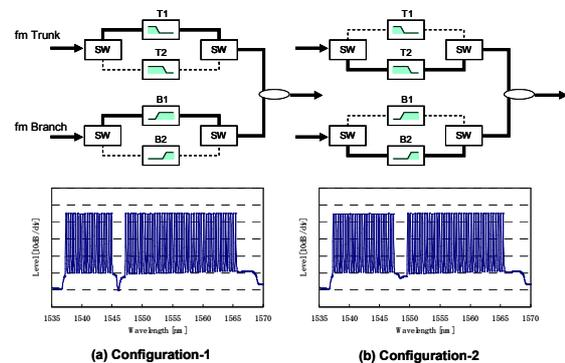
Figure 4: Optical Spectrum in each ROADM Configuration
