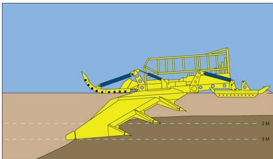
**Figure 4.** Rigid plow encountering a hard subsurface layer. Maintains deeper burial.
