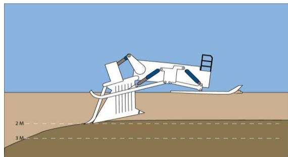
Figure 3. Articulated plow encountering a hard subsurface layer. Reduced burial results.
