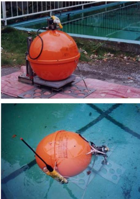
Fig6 Pop-up type seismometers
