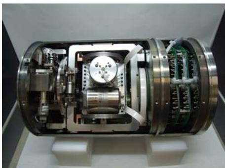
Fig.9 External view of seismometer
