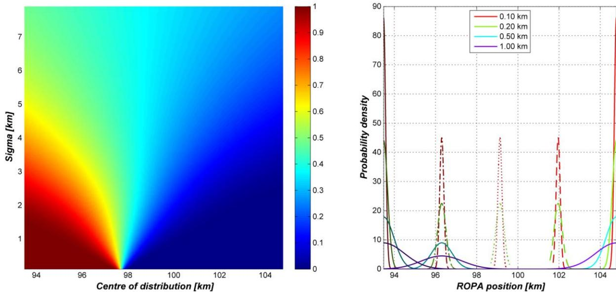
**Figure 7:** Failure probability of the link versus standard deviation and centre of the distribution for the ROPA position after fibre repair for the upgrade scenario to 40 Gbit/s CP-QPSK (left side). On the right side, some examples for the distribution are shown.
