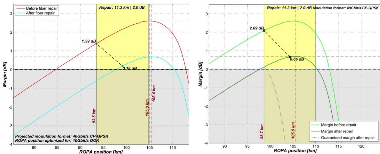
Figure 3: OSNR margin of a 40Gbit/s CP-QPSK channel versus ROPA position for system upgrade (left side) and greenfield application (right side). The upper curve shows the situation at begin of life (BOL), whereas the lower curve shows the remaining system margin after fiber repair.
