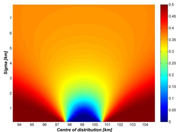
**Figure 8:** Average failure probability for the upgrade to 40Gbit/s CP-QPSK for bidirectional communication.
