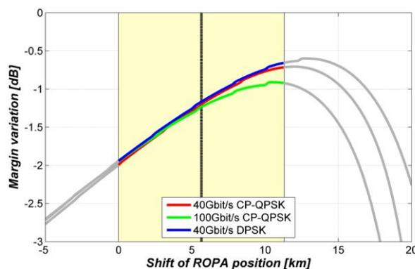
**Figure 5: Margin variation versus shift of ROPA position for different modulation formats.**
