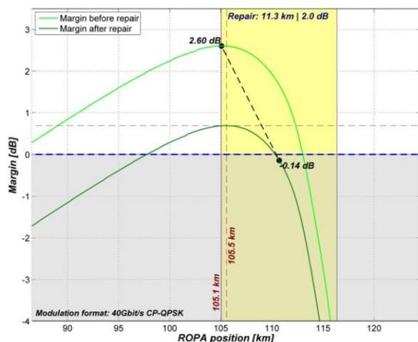
**Figure 4: Bad example: initially, the ROPA cassette is set to the position providing maximum margin at BOL.**
