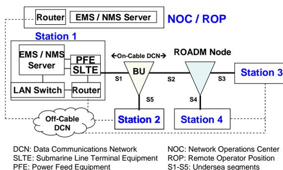
Figure 1 - Example Submarine Cable System EMS/NMS equipment and network architecture
