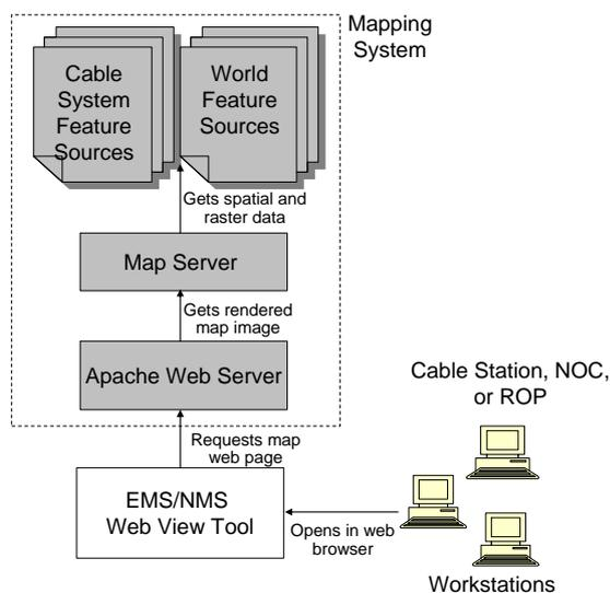
Figure 3 - Top Level Mapping Architecture
