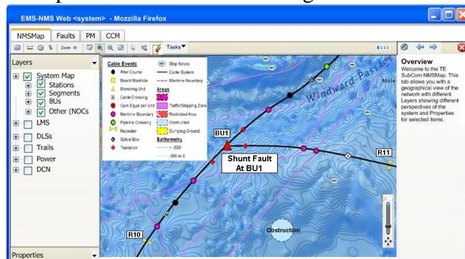
Figure 2: Example GIS-based Network Map Display
