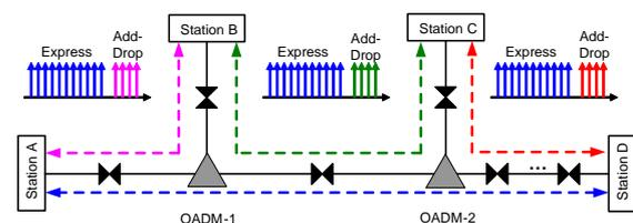
Fig. 1 – Typical  $\pi$ -network topology with two OADM nodes.
