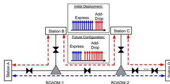
Fig. 2 –Agile  $\pi$ -network topology with two ROADM nodes. The ROADM nodes can be flexibly and remotely reconfigured based on traffic demand to accommodate increasing add/drop band to express band ratio, or to re-route individual wavelengths.
