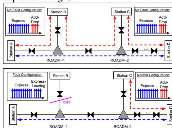
Figure 3. ROADM reconfiguration for node 1 in the event of a cable cut in the B branch: wavelengths previously routed through the B-branch are re-assigned to the trunk as express traffic. Top picture shows the normal (i.e. no fault) configuration, bottom picture shows the configuration in the event of a cable fault in segment B. Further, Station A can supply the express-loading as indicated in the box 'Fault Configuration'.
