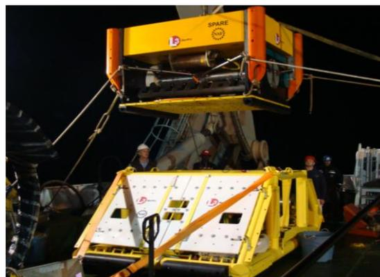
Figure 3: SIA Being Installed into a BIA
