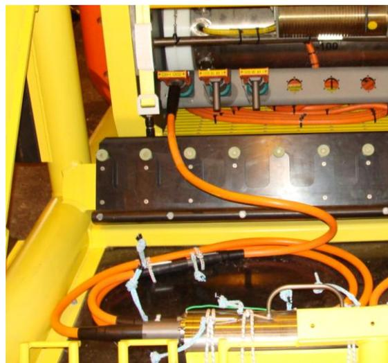
Figure 6: CSH Mounted on Node and Connected to SP1
