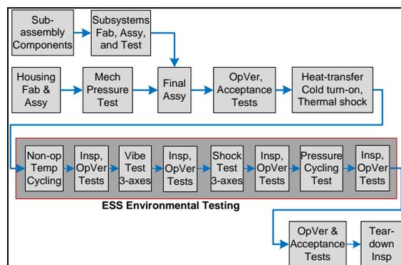
**Figure 9: Typical Qualification Test Flow**
