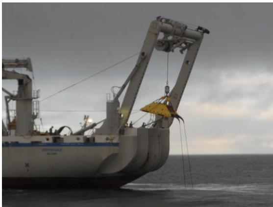
**Figure 11: Node Installation from TE SubCom Cable Ship CS DEPENDABLE**
