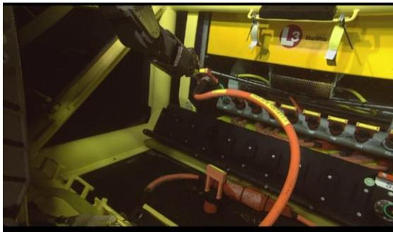
Figure 10: Subsea ROV Compatibility Testing
