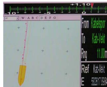
Fig 5: Logging of cable and ship position. Solid red line shows pre-defined route. Red squares show guide-weight position and yellow line show ship's position. Top left shows that cable position is 1.1 m off route.
