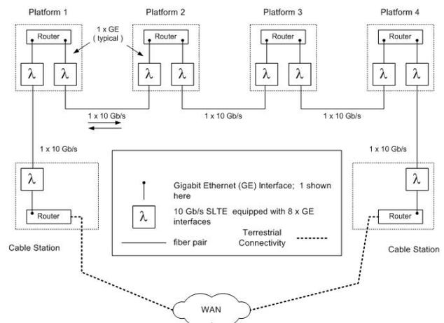
Fig. 4. Daisy-Chain Repeaterless Network
