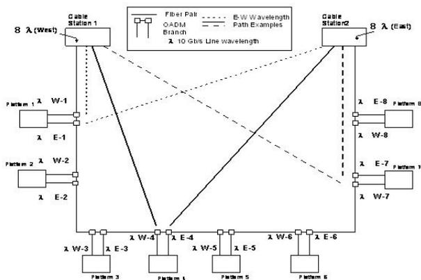
Fig. 5. Offshore network using Broadband OADM
