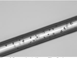
Figure 3 Compression Artifacts on Fiber Coating
