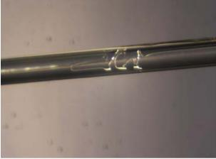
Figure 1: Coating Delamination
