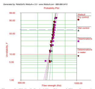
Figure 2: Weibull Probability Plots of Fiber Strength Data
