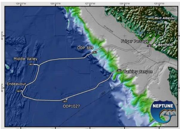
Figure 1. NEPTUNE Canada Cabled Ocean Observatory Proposed System Layout
