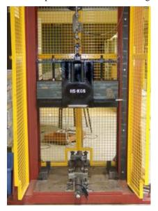
It consists of a substantial metal framework, bolted firmly to a concrete reinforced floor. A metal cradle, the weight of which can be adjusted between 115kg and 416.6kg in increments of 20.1kg by the addition of metal plates, is allowed to drop freely between greased uprights. The cradle can be raised to any desired height within the range 0 to 1.4m by an electric winch. The maximum impact energy the apparatus can therefore deliver is given by the formula
