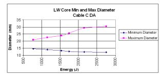
By doing so, it can be seen that the predicted impact energy level which caused the failure in these cases was approximately 750J or less. Electrical failure, or zero insulation thickness, was predicted by impact testing at 1723J. So the use of impact testing to predict actual energy levels for failure may not be appropriate, although with only two instances examined, more work needs to be carried out in this area.
