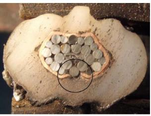
2) On several other cable types, especially those with high density polyethylene insulation, cracks and voids were seen at the higher energy levels. These would encourage electrical failure.
