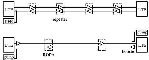
Figure 1: typical architecture of repeatered (top) and unrepeatered (bottom) transmission systems
