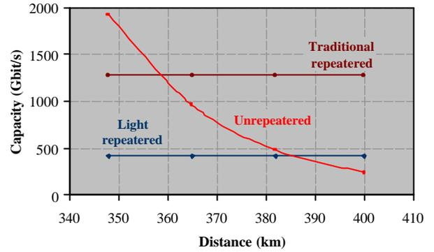
Figure 4: Capacity versus distance @ 10 Gb/s (constant margin)
