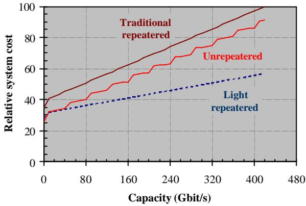
Figure 3: Relative system cost for a 10 Gbit/s line rate
