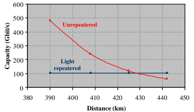
Figure 3: Capacity versus distance @ 2.5 Gb/s (constant margin)
