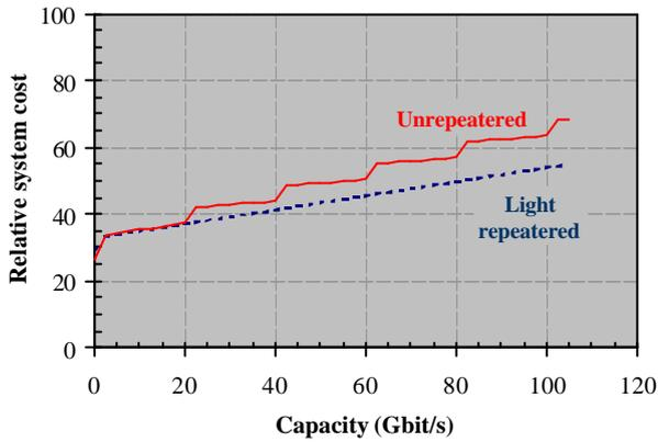
Figure 2: Relative system cost for a 2.5 Gbit/s line rate
