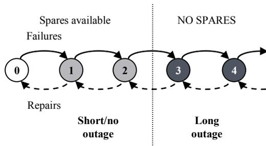
Figure 3: Example state diagram for the case of a location with 2 spares
