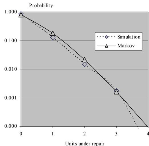
Figure 4: Comparison of Simulation and Calculation
