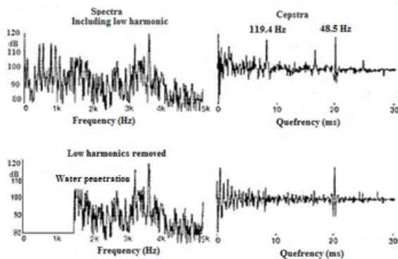
Fig.3 The spectrum from a subsea fiber optic cable structure in its deteriorated condition
