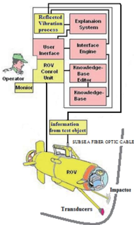
Fig. 1. The most important modules of proposed rule-based vibration signal diagnostic expert system
