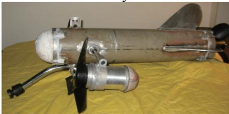
Fig.2 The proposed ROV and diagnostic arm
