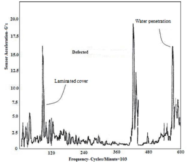
Fig.5 Frequencies below that of half of the Impactor frequency are removed - faulty subsea cable
