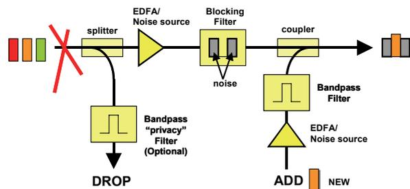
Figure 13: Effect of Trunk Failure on Active OADM BU
