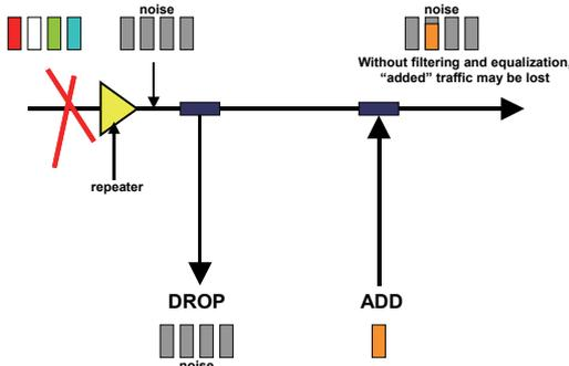
Figure 11: impact of a trunk fault on added traffic
