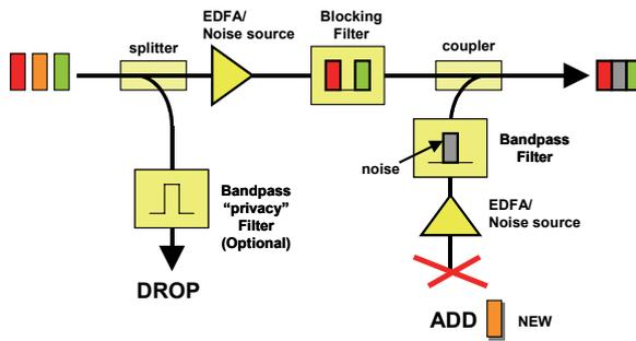
Figure 14: Effect of Branch Failure on Active OADM BU
