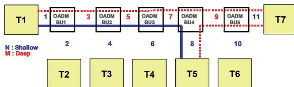
Figure 5: DLS T1-T5 path with OADM (Short route in blue, long route in red)
