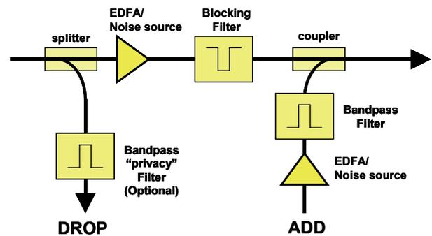
Figure 12: Active OADM Branching Unit Optical Block Proposal
