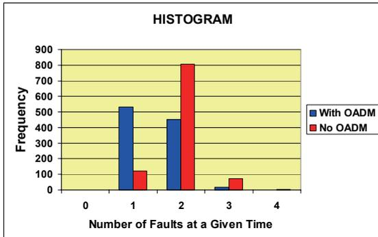
Figure 7: Probability distribution for the occurrence of simultaneous failures in 10 years for DLS T1 to T5, with and without OADM, simulated
