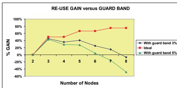
Figure 10: Bandwidth gain of “OADM with bandwidth re-use” versus “wideband OADM”, versus number of nodes and guard band size, for equally distributed DLS capacity
