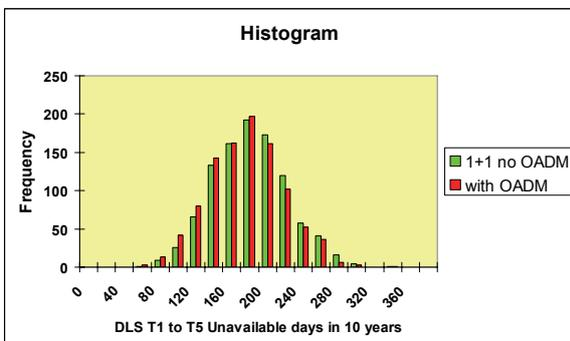
Figure 8: OADM versus non-OADM 1+1 internal restoration, simulated (with express fibre pair)
