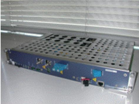
Figure 3: DPSK Transponder Card
