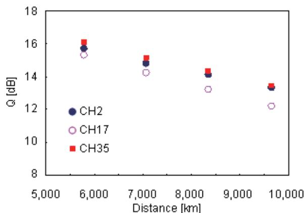
Figure 7: Q Factors vs. Transmission Distance
