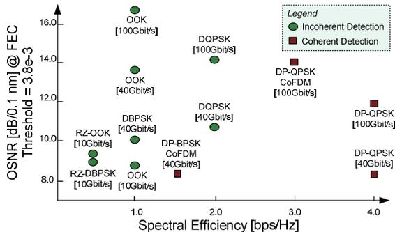
Figure 1. 40G/100G Modulation Comparison
