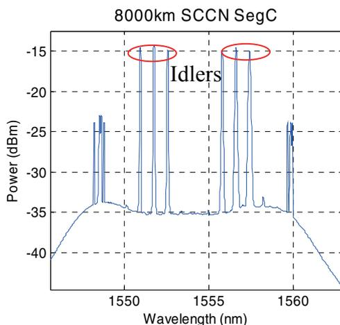
Figure 7. 8000km SCCN Segment C Receive Spectrum- Blue Band Testing
