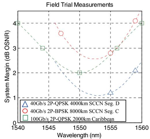
Figure 8. Measured Net System Margin for 40G/100G technology on Dark Fiber
