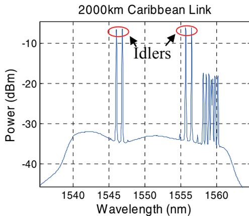
Figure 6. 2000km Caribbean Link Receive Spectrum – Red Band Testing
