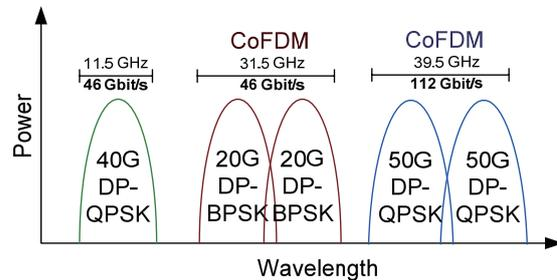
Figure 3. 40G/100G DP-PSK Spectral Occupancy
