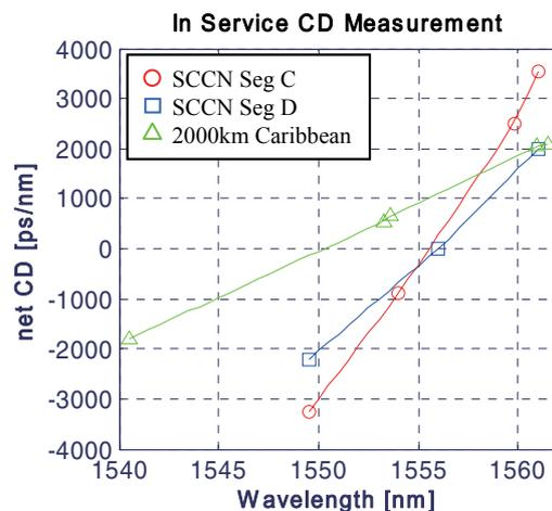
Figure 5. In-Service CD Measurements
