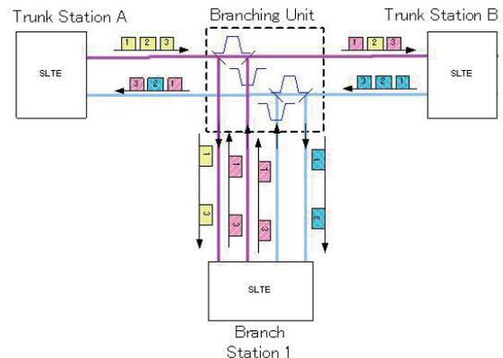
**Figure 2: OADM system using submersible BU**
