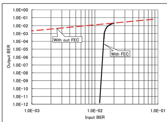
**Figure 4: Error correction performance of the FEC function**
