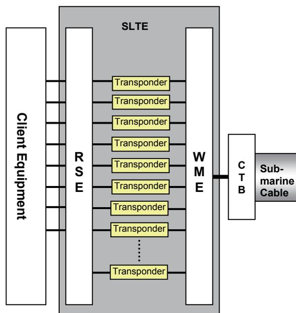
**Figure 1: Main function blocks of SLTE**
