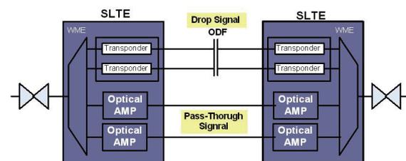
**Figure 3: OADM system using pass-through scheme in SLTE**
