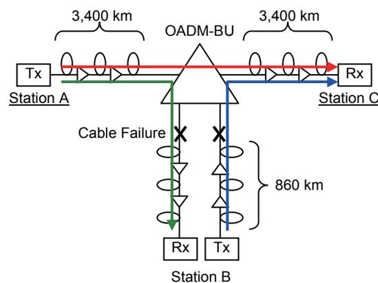
**Figure 4: Demonstration Setup**
