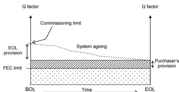
Figure 1 Main parameters from the Power Budgets. The dash line means that no linear assumption can be made on failure/cable cut occurrences over time.
