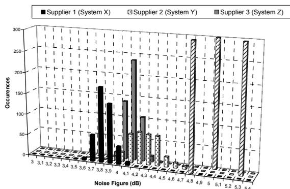
Figure 2 Comparison between Power Budget assumption and noise figure measured during the repeater tests in the factories
