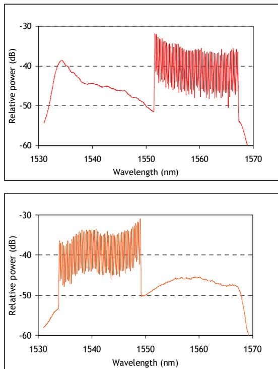
**Figure 10 : Pair #2 Received 58-channel Spectrum with Cable Cut in the OADM BU Section on the Branch (Top) – Pair #2 Received 58-channel Spectrum with Cable Cut in the OADM BU Section on the Trunk (Bottom)**
