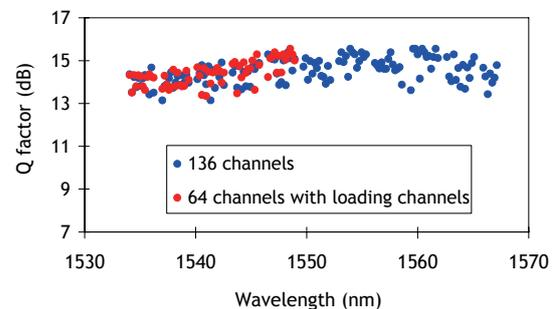
**Figure 4 : 5800 km Transmission Performance - Q Factor of 136 Channels in Blue - Q Factor of 64 Channels with Loading Channels in Red**
