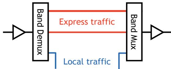
**Figure 2 : Example of Band Multiplexing in Intermediate SLTE Station**
