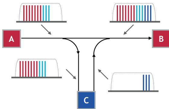
**Figure 5 : No Wavelength Re-use BU Scheme (Express Channels in Red, Drop Channels in Light Blue, Add Channels in Dark Blue)**
