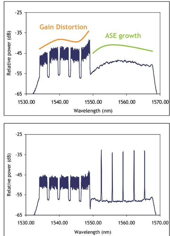
**Figure 3 : Received Spectrum after 5800 km with Partial Loading (top) and with Loading Channels Lit Up (bottom)**
