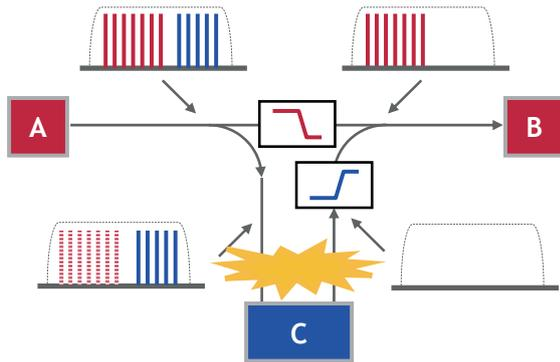
**Figure 7 : System Loading in Case of Cable Cut in Shore-end Section of Intermediate Station**
