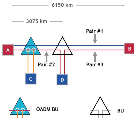
**Figure 8 : Express Fibre Pair: Pair #1 – Omnibus Fibre Pair (with OADM BU): Pair #2 – Omnibus Fibre Pair (No OADM BU): Pair #3.**
