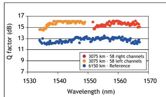
**Figure 11 : Pair #1 Q Factor for Full Multiplex in Blue - Pair #2 Q Factor in Red (58 Channels at Longest Wavelengths) - Pair #2 Q Factor in Orange (58 Channels at Shortest Wavelengths)**
