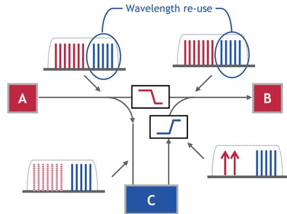
**Figure 6 : Wavelength Re-use BU Scheme (Express Channels in Red, Drop Channels in Blue, Add Channels in Blue, Red Arrows Represent Loading Channels)**
