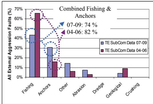
Figure 2b. Combined Comparison of Fishing & Anchor Faults for all Water Depths
