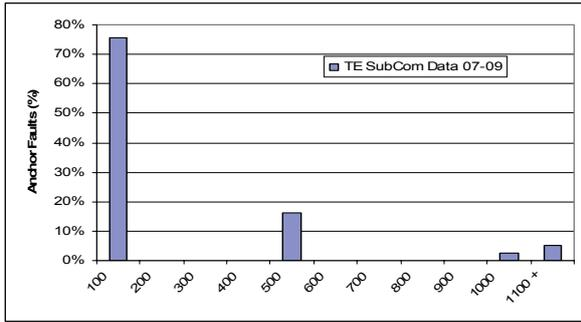
Figure 4b. Water Depth Distribution (m) of Anchor Faults
