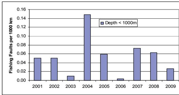
Figure 7. Length-Normalized Fishing Faults in less than 1000m Water Depth
