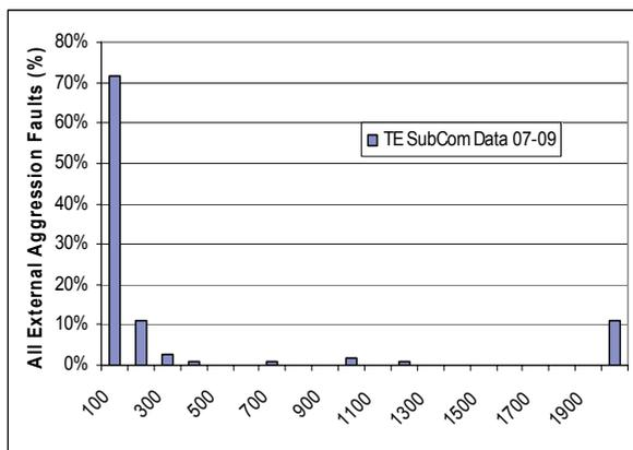
Figure 3a. Depth Distribution (m) of all External Aggression Faults
