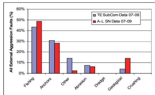
Figure 2. External Aggression Faults for all Water Depths
