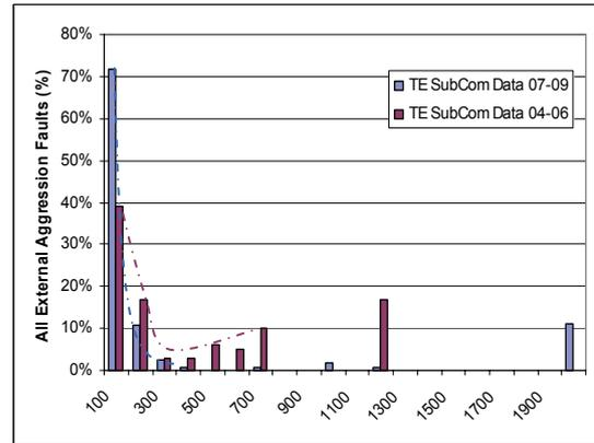
Figure 3b. Depth Distribution of All External Aggression Faults Comparing (2) time periods
