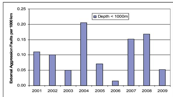
Figure 6. Length-Normalized External Aggression Faults in less than 1000m Water Depth
