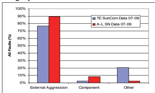
Figure 1. Overall Causes of Fiber Optic Cable Failure
