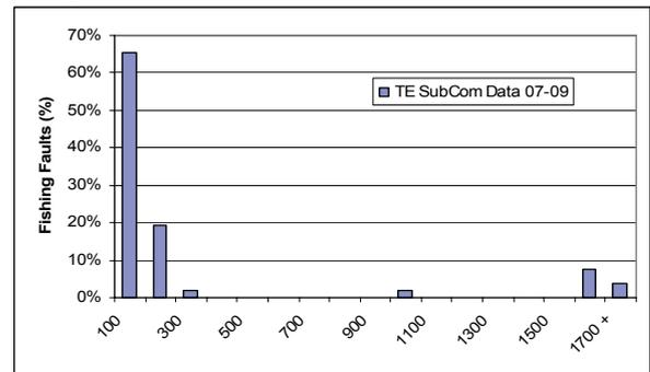
Figure 4a. Water Depth Distribution (m) of Fishing Faults
