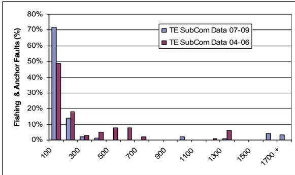
Figure 4c. Water Depth Distribution (m) of Fishing & Anchor Faults
