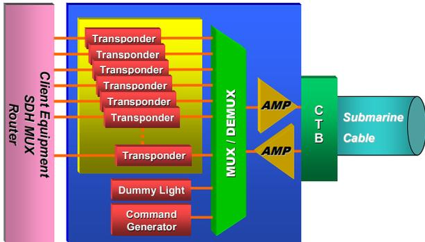
**Figure 1: Functional block diagram of SLTE**
