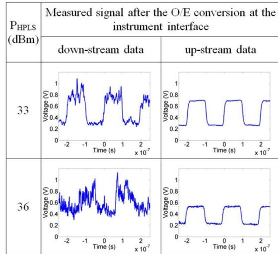
**Figure 2: Examples of the transmitted data obtained after the O/E conversion for two cases of the HPLS optical power supply, respectively set at 33 dBm and 36 dBm.**
