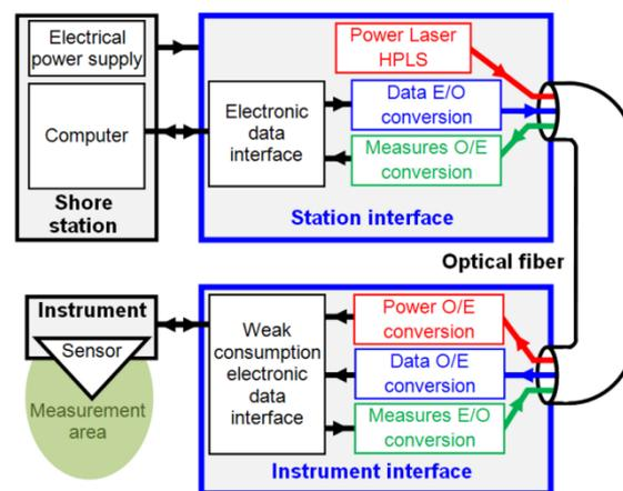
Figure 1: Schematic of the quasi-all-optical architecture.
