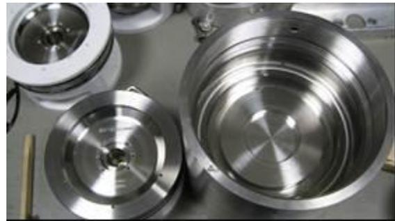
**Figure 16: demountable bulkhead sealing system**
