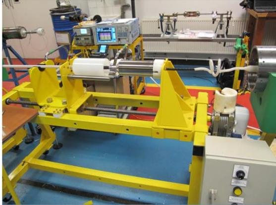
**Figure 12. Multi-function jointing frame**
