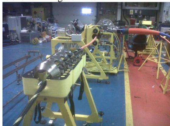
**Figure 11. Cable integration packs and new in line armour press being used on a titanium branching unit**
