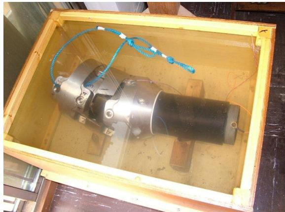
**Figure 2. Termination /coupling cell corrosion test**
