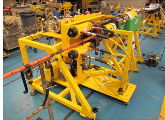
**Figure 14. In-line armour press in action**
