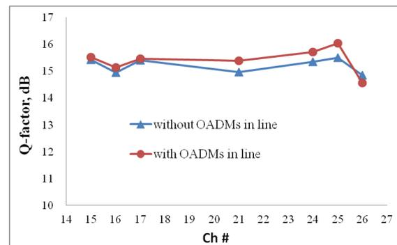
Figure 6: Q-factor performance for service channels with and without OADMs
