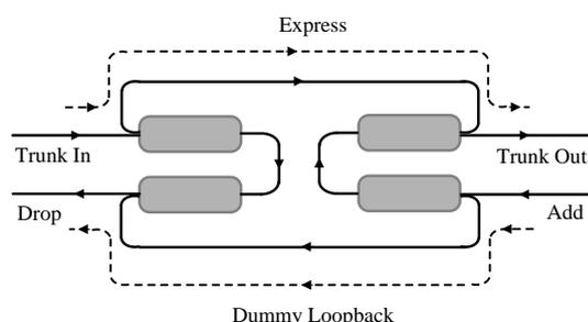
Figure 1: TFFs based OADM configuration
