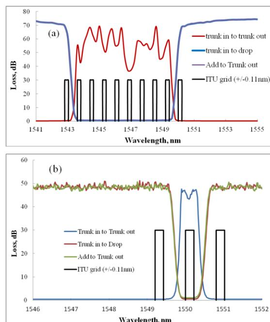
Figure 2: Loss spectra of OADM modules (a) 100GHz 8s0 (b) 100GHz 1s0
