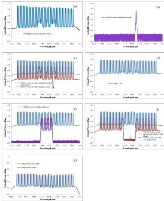
Figure 5: Optical spectra measured in different positions of the link
