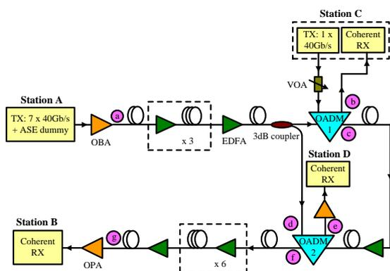
Figure 3: Transmission experimental setup
