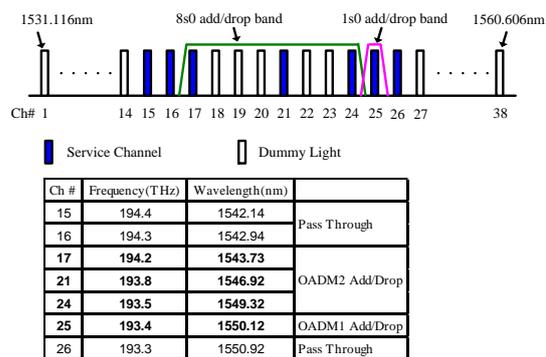
Figure 4: Wavelength allocation of service channels
