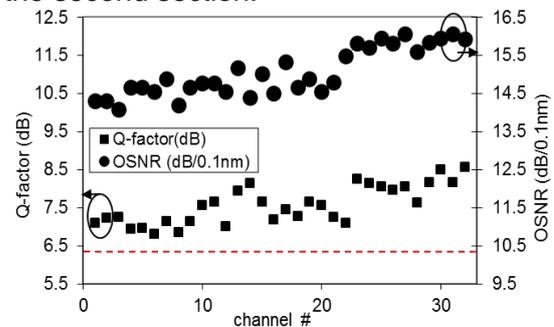
Figure 7: Received OSNR (in 0.1nm RBW) and Q-factor for all 120-Gb/s PDM-QPSK channels after 445-km
