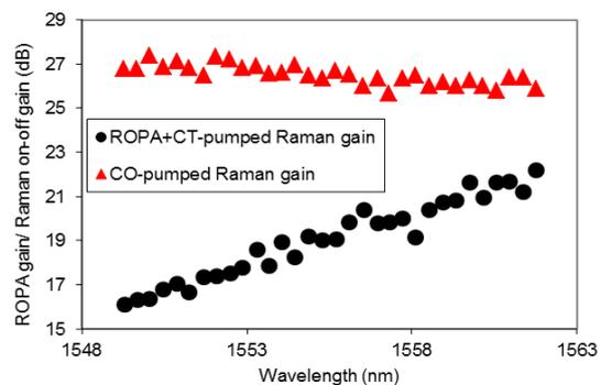
Figure 6: The measured on-off co-pumped Raman gain in the first section and net gain from ROPA/1480nm Raman gain in the second section.
