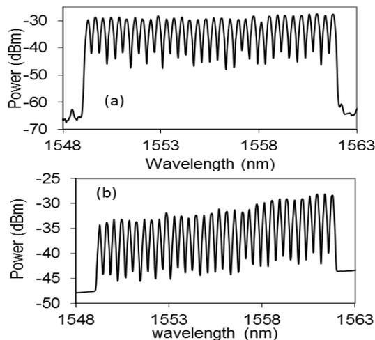
Figure 5: Transmitted (a) and received (b) optical spectra of DWDM 120-Gb/s channels after 445-km transmissions
