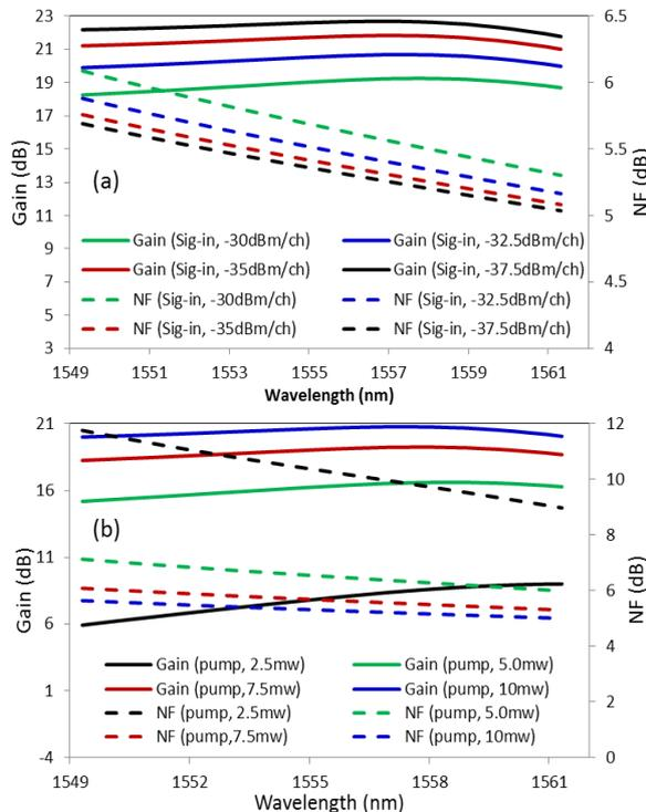
Figure 3: Simulation result of the gain and NF of ROPA
