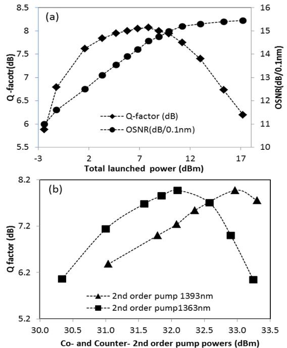
Figure 4: (a) Q-factor and received OSNR of center channel vs. total launch power when the co and counter 2nd pump power were fixed at optimum levels; (b) Q-factor
