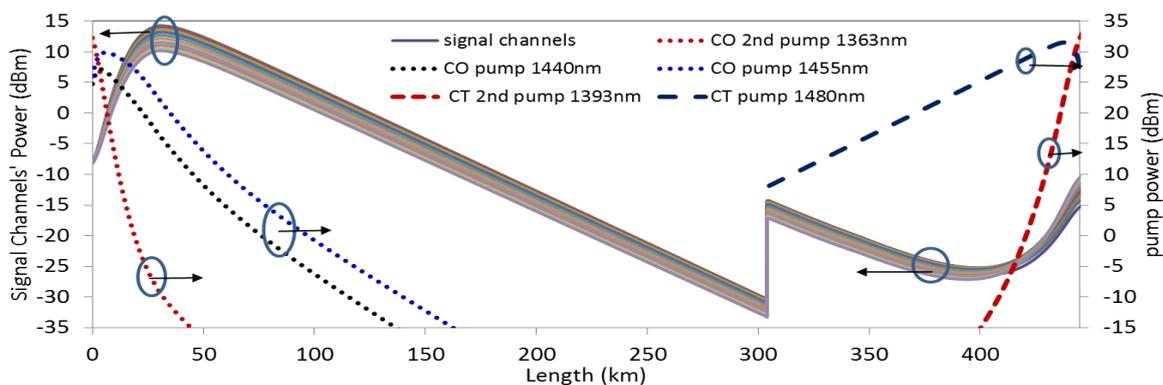
Figure 2: Simulation result of optical powers for the WDM channels and pumps evolution along the fiber line under optimized conditions
