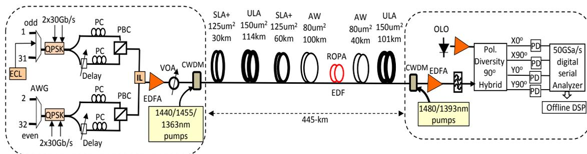
Figure 1: Schematic diagram of experimental setup for unrepeated transmission system.
