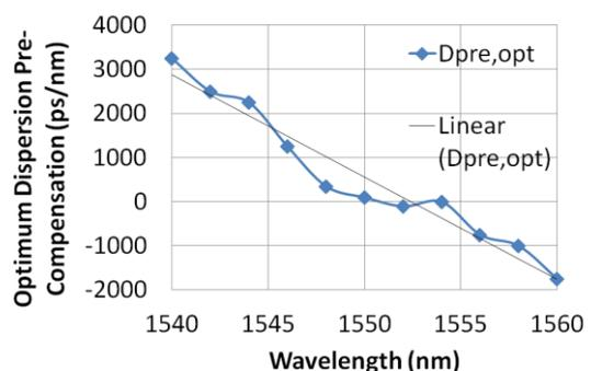
**Figure 4: Optimum dispersion pre-compensation as a function of wavelength for 100 Gb/s CP-QPSK WDM signals with 50 GHz of channel spacing at the optimum power of -5 dBm over 4000 km.**
