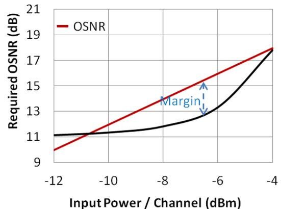
**Figure 2: ROSNR as a function of input power / channel for 40 Gb/s CP-QPSK WDM signal with 50 GHz channel spacing at 1550 nm over 6000 km with optimized pre-compensation.**
