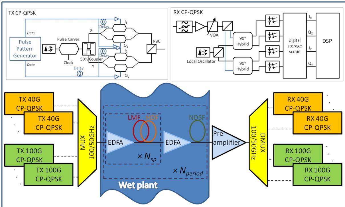
**Figure 1: Setup of the investigated multi-span submarine system. Inset left hand side top: Setup of transmitter of CP-QPSK signal. Inset right hand side top: Coherent Receiver.**
