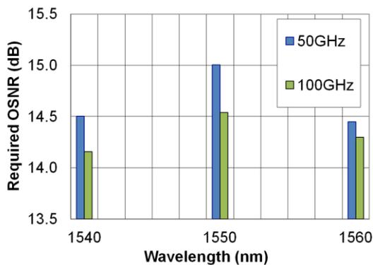
**Figure 3: ROSNR as function of the wavelength for 100 Gb/s CP-QPSK WDM signal with 50 and 100 GHz of channel spacing at the optimum pre-compensation and launch power of -5dBm over > 4000 km.**
