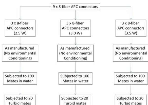
**Figure 6:** High Optical Power Test Flowchart
