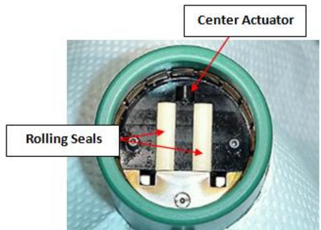
**Figure 2:** The current optical wet-mate design, which comprises three actuators, one for each Rolling Seal in the fixed connector and one for both seals in the flying connector
