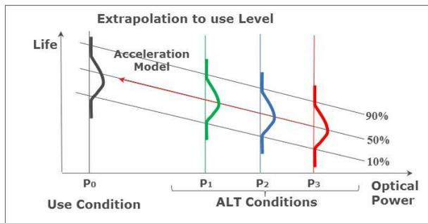
**Figure 9:** Accelerated Life Testing Methodology
