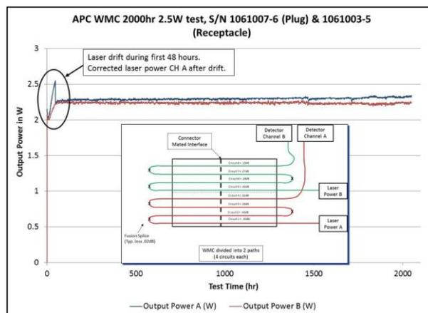
**Figure 8:** Test data from first 2000 hour high optical power test performed
