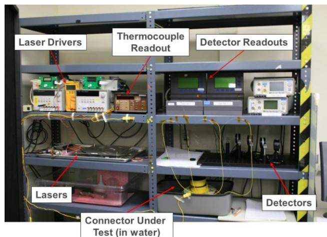
**Figure 7:** Test setup for single 8-fiber wet-mate connector high optical power test
