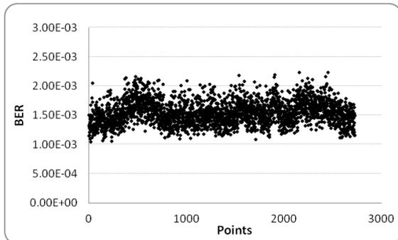
Fig 9: Long term BER monitoring data, the two points' interval is 30s
