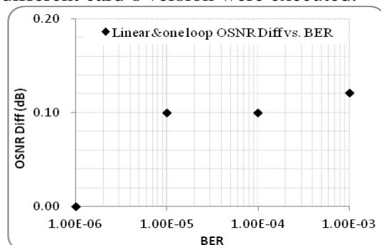
Fig 6: OSNR difference between on-line adapted and commercial version versus BER for 31x46Gb/s at 100GHz transmission over 1139km straight line and one loop system
