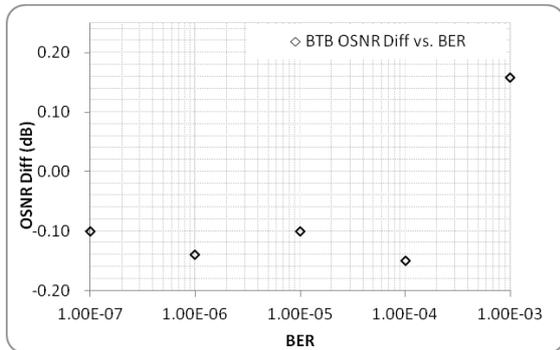
Fig 3: OSNR difference between on-line and commercial version versus BER
