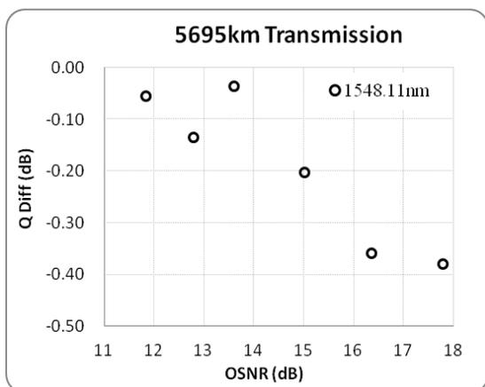
Fig 7: OSNR vs. Q difference after 5695km system transmission after five loops for off-line and on-line testing mode
