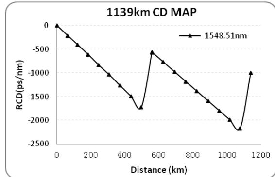
Fig 4: CD map for the 1139km loop link
