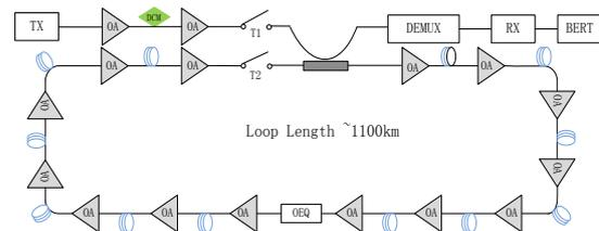
Fig 5: Loop system setup
