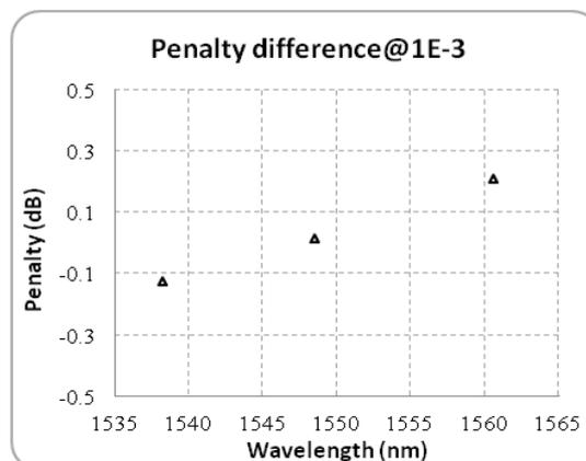
Fig 9: The penalty difference between on-line and off-line testing mode after 6600km system transmission
