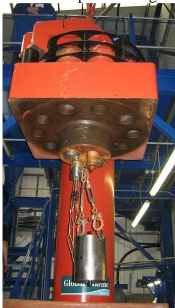
**Figure 14: Test sample is attached and connected to the pressure vessel lid**
