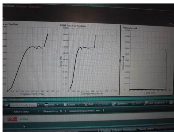
**Figure 2: The two left hand graphs show a dip in load suggesting a failure. The right hand graph shows a catastrophic leak.**
