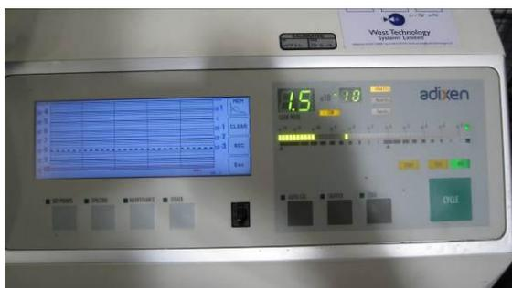
Figure 17: Helium leak rate
