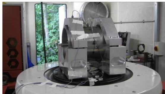
**Figure 12: Bump and vibration testing**
