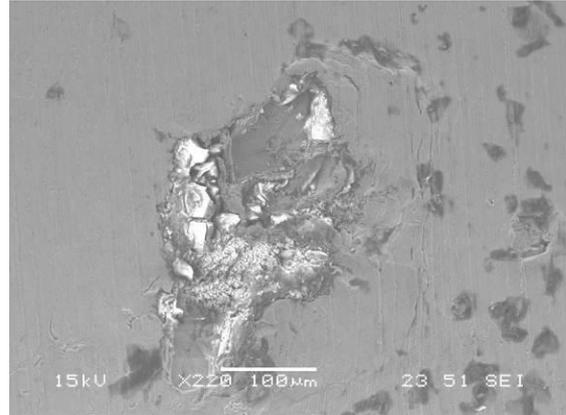
**Figure 5: Aluminium Oxide contamination from a cleaning process**
