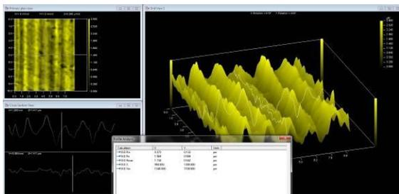
**Figure 9: Laser scan measurement of the Bulkhead main sealing surface.**
