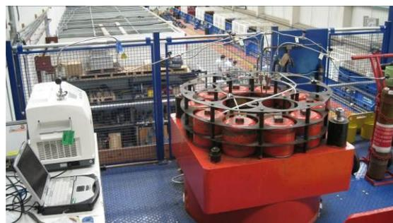
**Figure 15: Test sample is connected to the helium leak detector (left) and helium source (right)**
