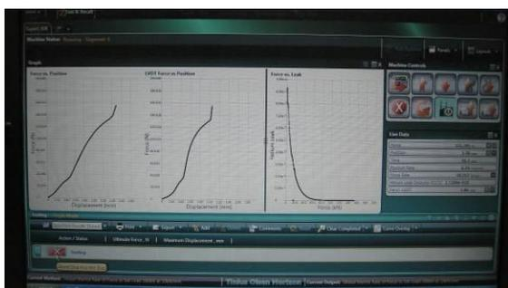
**Figure 10: Load v's displacement of press and bulkhead, plus leak rate v's load**
