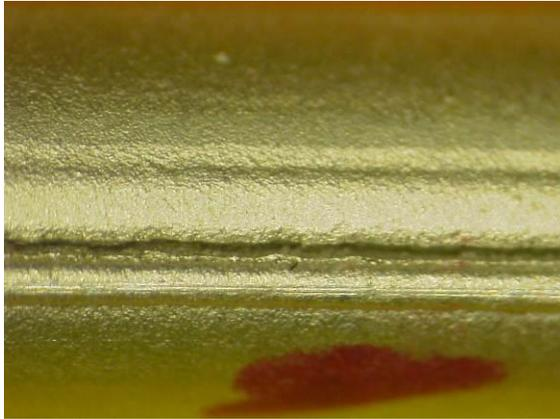
**Figure 3: The photo reveals a possible tear in the plating**
