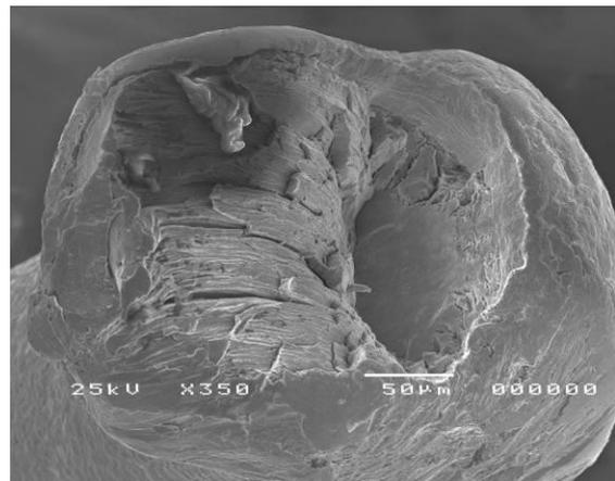
**Figure 6: Typical green fracture**
