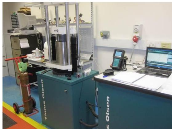
**Figure 1: Test equipment including hydraulic press, leak detector, helium source and data logger.**
