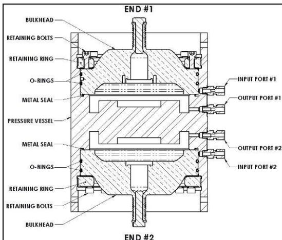
**Figure 11: Test assembly section view**
