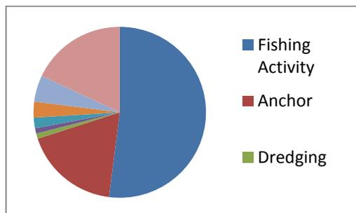
**Figure 1 – Causes Of Cable Damage**
