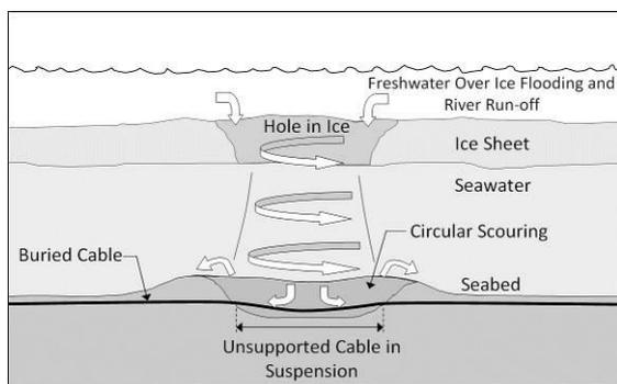
Figure 7 Strudel Scour Process and Cable Suspension
