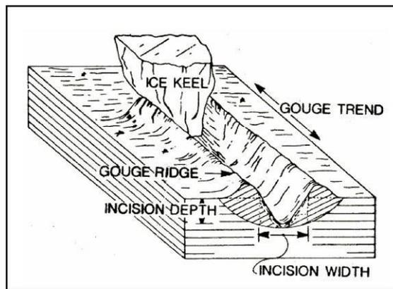
Figure 5 Illustrated Single Keeled Ice Gouge Characteristics
