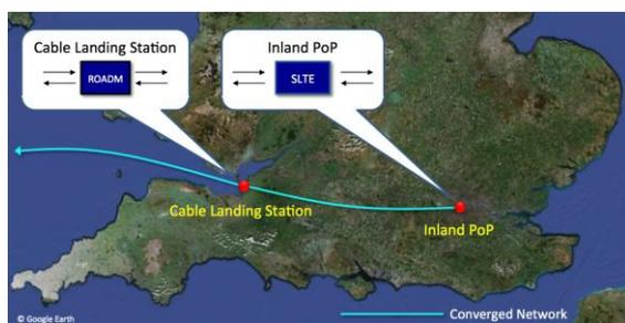
**Figure 3: Converged Global Network by Leveraging Photonic Cable Landing Stations**
