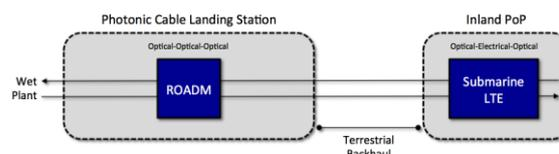
**Figure 2: Photonic Cable Landing Station Transport Network Elements**
