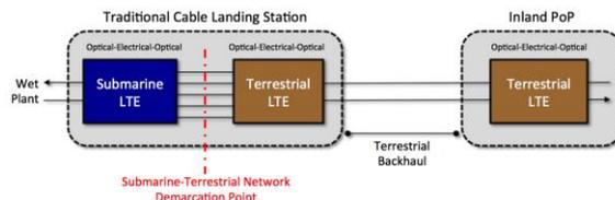
**Figure 1: Traditional Cable Landing Station Transport Network Elements**
