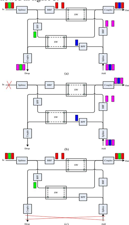
Figure 3. (a)OADM with bypass function, (b) Light flow of trunk fault recovery, (c)
