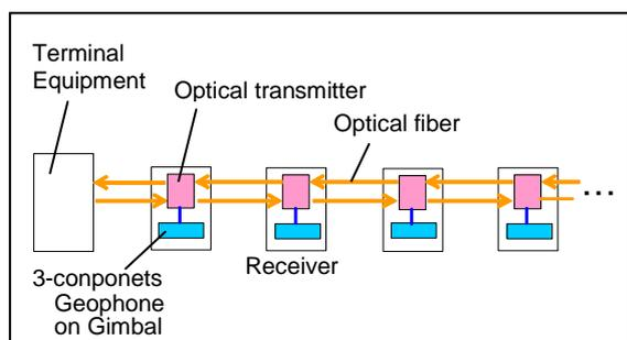
Figure 1: Conventional RSCS data transmission schema
