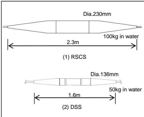
Figure 4: Comparison of RSCS and DSS receiver size
