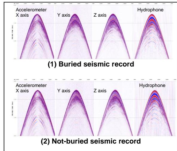
Figure 10: Seismic records comparison of DSS receiver buried and not-buried
