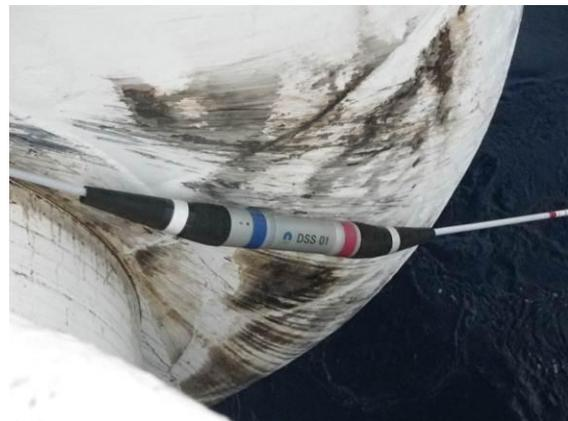
Figure 7: DSS receiver deployment
