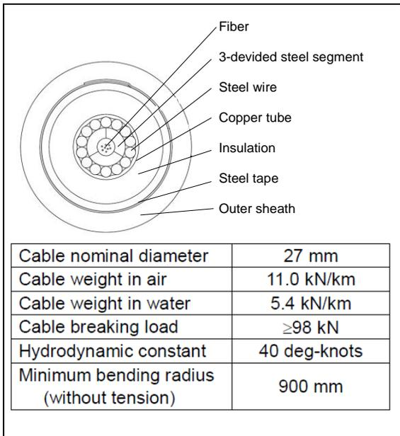
Figure 5: Optical submarine cable (OCC-SC300-LWS)
