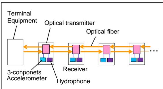
Figure 6: DSS data transmission schema
