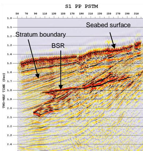
Figure 3: BSR reflection record obtained by RSCS in 2006
