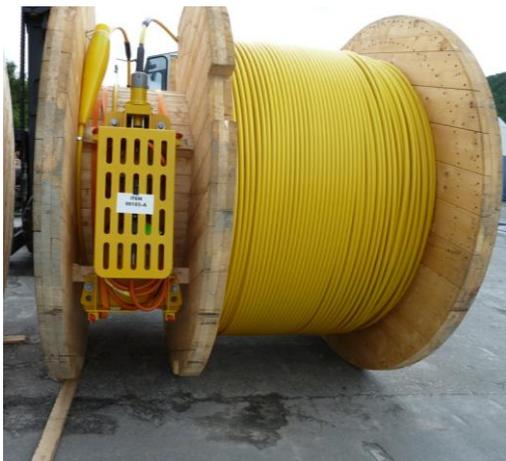
**FO cable with CEM with wet mate connector.**
